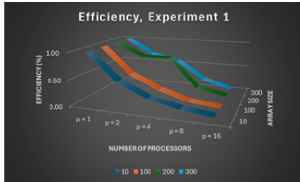
Figure 4: A line graph displaying the calculated efficiency for each array size for a given number of processors for experiment 1.
